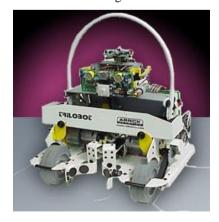
Figure 2. Trilobot (Arrick Robotics, USA) experimental robot
